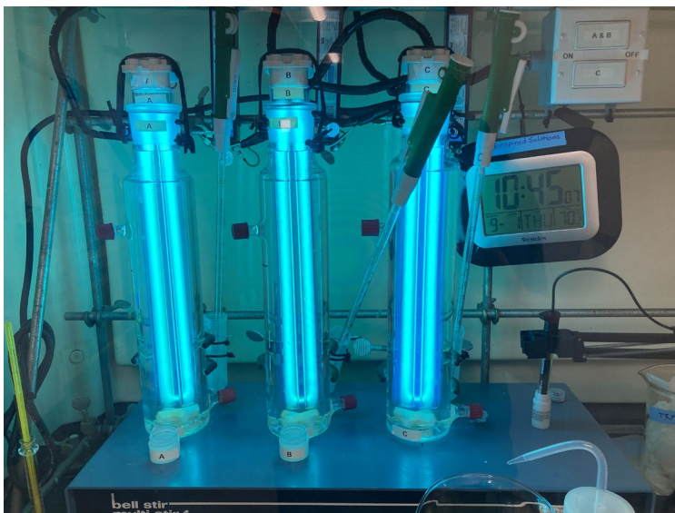
Figure 3-1. Benchtop test reactor set up for small scale treatability studies.
