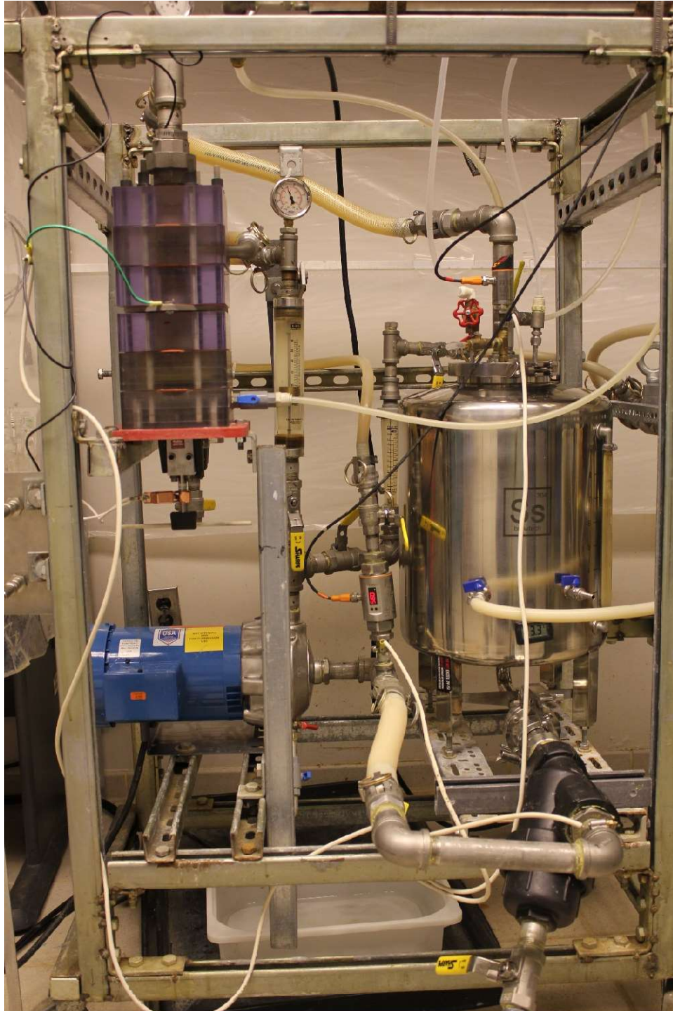
Figure A-3. Photograph of Onvector's Laboratory Plasma Destruction System (AC Power Supply and Vacuum Pump not shown).
