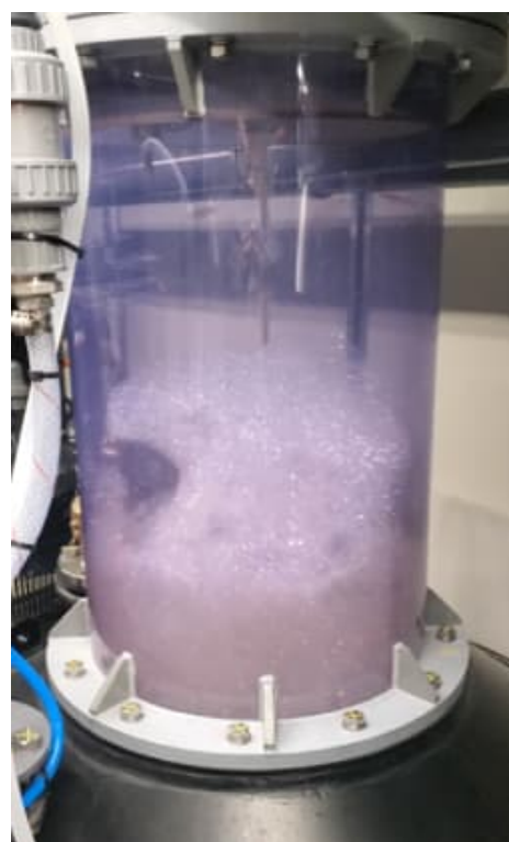
Figure E.16: Shakopee Aquifer Secondary Fractionation Foam Production.
