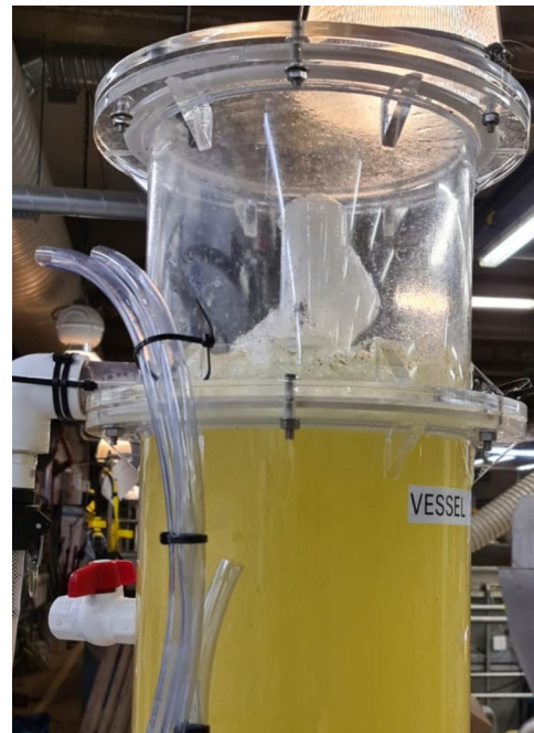
40-ft OPEC system for landfill leachate treatment in Sweden
